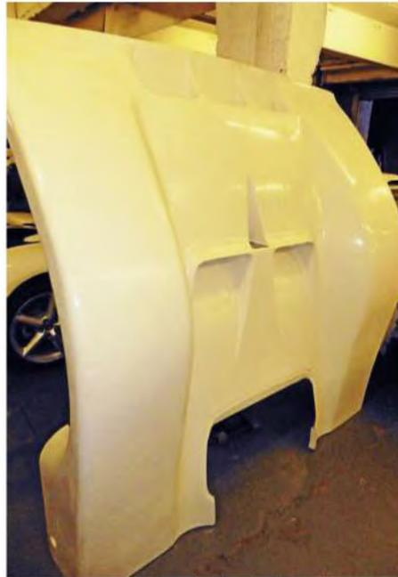
Dummy front ends produced to test original mould
