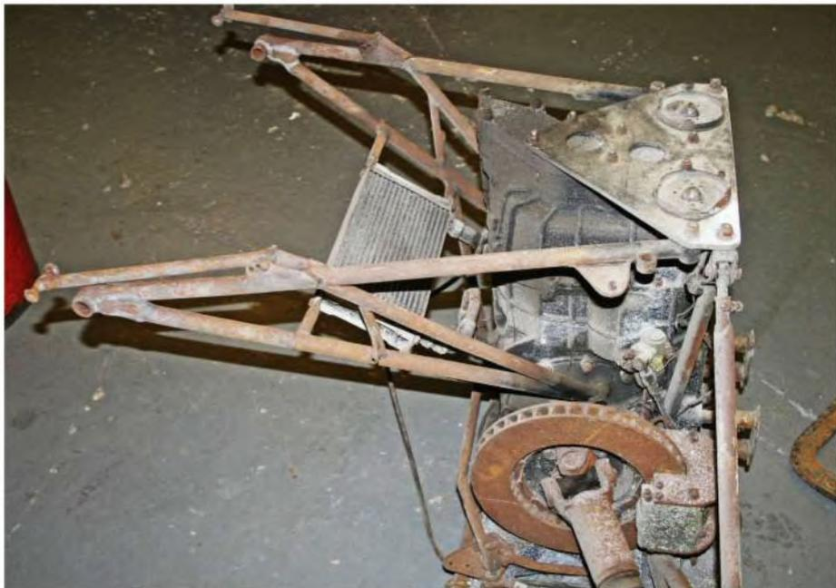
Not a lot to go on - the rear subframe and transaxle as dragged out of storage
