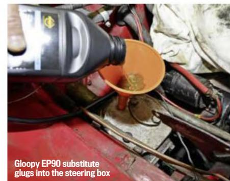
Gloopy EP90 substitute glugs into the steering box
