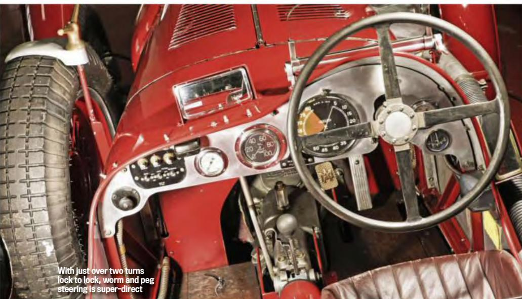
With just over two turns lock to lock, worm and peg steering is super-direct
