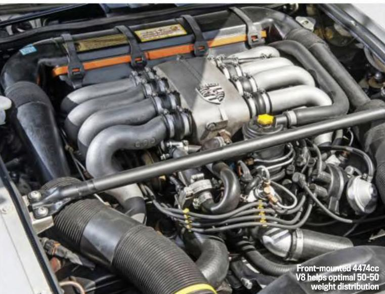
Front-mounted 4474cc V8 helps optimal 50-50 weight distribution
