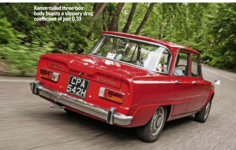
Kamm-tailed three-box body boasts a slippery drag coefficient of just 0.33
