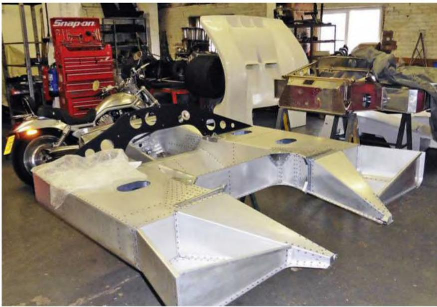
Body tub had to be completely repanned because bonding had failed - not great when up against the clock
